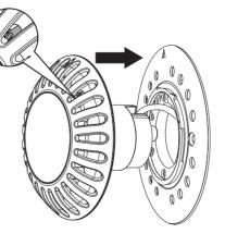
2 ROTATE LIGHT CLOCKWISE TO LOCK INTO POSITION
