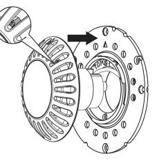
**ROTATE LIGHT CLOCKWISE TO** LOCK INTO **POSITION**
